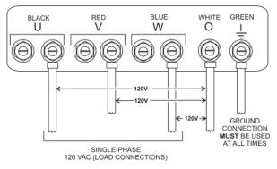
Figure 22. UVWO Terminal Lugs 1Ø-120V Connections
